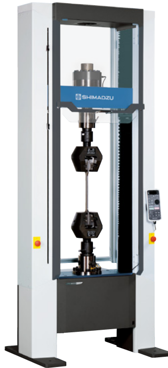
AGS-300kNX2 + 300kN Non-Shift Wedge Type Grips
